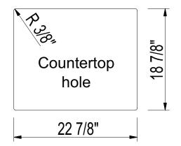
**NOTES:** Refer to installation instructions supplied with kitchen sink for undermount, or drop-in installations. Templates and installation kits provided with the sink.
